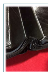
24 ply 0.5mm PEKK w continuous C fibers
